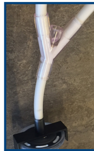
Photo 16 - Duo adapter allows a single bag to be used simultaneously by more than one vaccinator.
