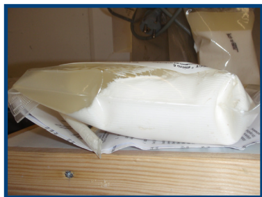
Photo 4 - Lying in refrigerator. Must be shaken before it is ready for use (oil on top)
