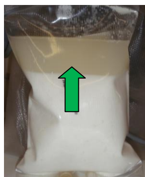
Picture 2 Oil on top during storage is normal
