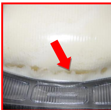
Picture 3 Broken emulsion -do not use
